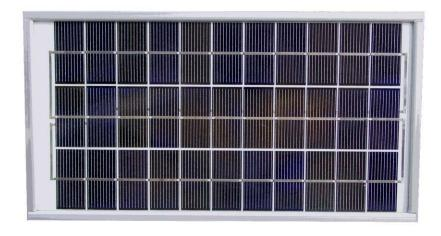
The FASM6 solar panel may be used to power FA575 wireless repeaters and FA536 wireless locators in remote areas. The only modification necessary is to replace the standard 1.2 amp hour storage battery with a 4.0 amp hour battery. The solar panel is not suitable for use in very cold climates as an accessory heater is required for cold outdoor installations. In these instances one must find an AC plug for power.
